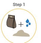
Prepare and apply mortar with cement - sand ratio of 1:4 on roof
